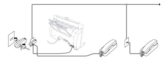
Whenever this external phone (or TAD) is in use, the screen displays **EXT. TEL IN USE**, and, if the MFC's handset is lifted, an alarm sounds. To disconnect the call on the external phone and switch to the MFC, lift the handset and press **Tel** (for MFC 730 only) or **Speaker Phone** (for MFC-740 only).
